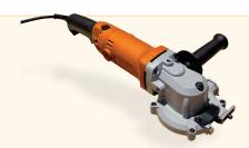
BNCE-20 The Original Cutting Edge Saw<sup>™</sup> A multipurpose cutting tool. It can easily cut #6 (3/4") rebar, all-thread rod, chain, EMT conduit, copper pipe, steel rods, steel tubing, and much more. This AC powered handheld tool is lightweight and features a three position handle. The capacity of the opening is .875" (23.62mm). This tool is ETL Listed and is excellent for cutting rebar or bolts near flush with concrete or block construction.
