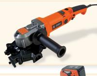
BNCE-30 Cutting Edge Saw™ A multipurpose cutting tool. It can easily cut #8 (1") rebar, all-thread rod, chain, EMT conduit, copper pipe, steel rods, steel tubing, and much more. This AC powered hand-held tool is lightweight and features a three position handle. The capacity of the opening is 1.18" (30mm). This tool is ETL Listed and is excellent for cutting rebar near flush with concrete or block construction.
